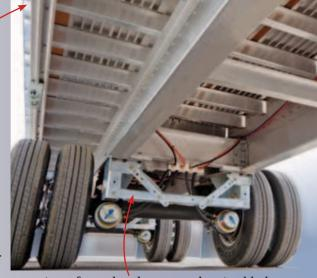
I beam floor sills provide superior strength.
