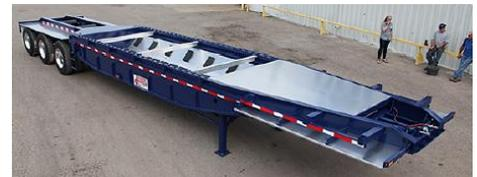
Coils can range in size from something relatively small like 5,000 lbs. to over 60,000 lbs. Doonan's new Flatbed Coil Hauler trailer's Gross Vehicle Weight Rating (GVWR) is 98,000#. The GVWR is based on a tri-axle trailer with disc brakes.
