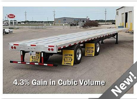
The Doonan® engineered Narrow Neck Platinum Flatbed Trailer has 3,870 CF of volume, based-off a 47" fifth wheel height. By comparison, a standard Flatbed Trailer has 3,701 CF of volume, based-off a 49" fifth wheel height. The difference results in a 4.3% gain in cubic volume in Doonan's custom-engineered design. Both calculations are based-off a 13' 6" overall height.
