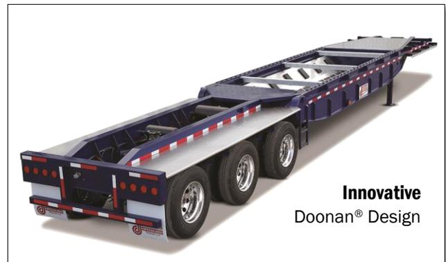
Coils are generally some of the toughest types of freight to haul because of their concentrated weight in one small area on the trailer. One of the many advantages of Doonan's trailer design is that Doonan® has engineered the coil well closer to the axles, in order to transfer more weight onto the trailer axles.
