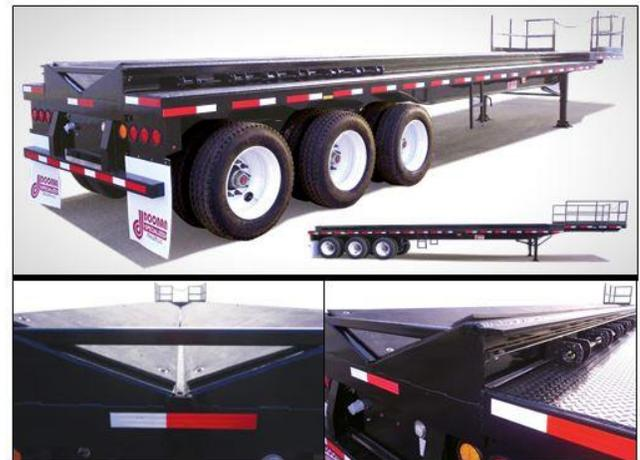
A convenient walkway on both sides of the channel allows for easy inspection of the load. Tie-downs can be applied by a driver from alongside the trailer to further support the securement of the coils, via a sliding winch track on both sides.
