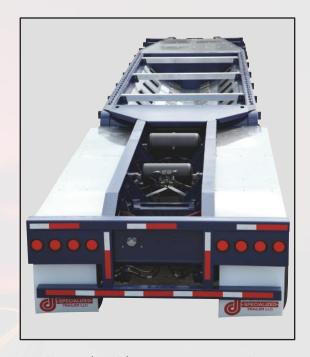
Engineered with two outer perimeter beams with 1" x 5" top and bottom flanges, the new Doonan® manufactured trailer features a well opening in the center that measures 19' long x 76" wide, with recessed concave beams to safely secure and haul 3' to 7' diameter coils.
